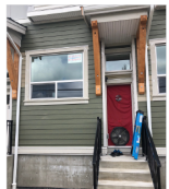
Image 2: Final blower door testing at multi-family townhouse project
