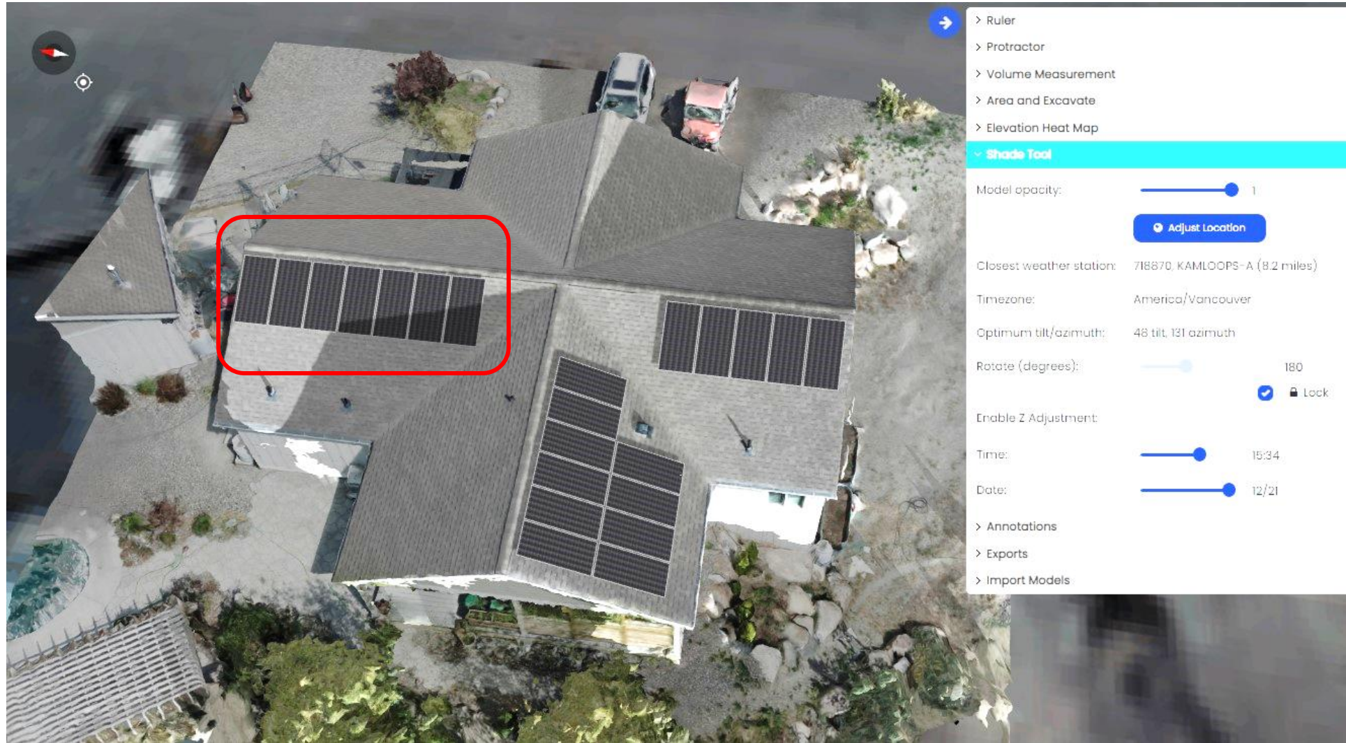
West Facing Array Shading by West Gable
